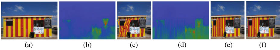
Fig. 1 Resizing with/without orientation information: a input image with vertically-biased features; b accumulated energy map using conventional gradient magnitude; c resizing based on b ; d accumulated energy map using horizontal gradient only; e resizing based on d ; f proposed method
