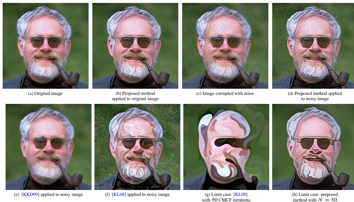
Figure 12: (a)-(f): Anisotropic Kuwahara filter, shape-simplifying image abstraction, and proposed method applied to an image corrupted with 2% Gaussian noise and 5% impulse noise. (g)-(h): Limit cases.
