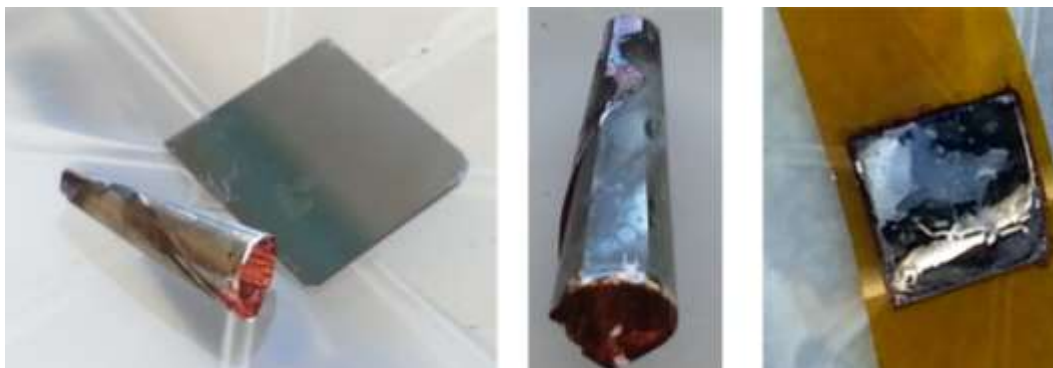
Figure 2.21: Problems with GaSb films- cracking and oxidation
