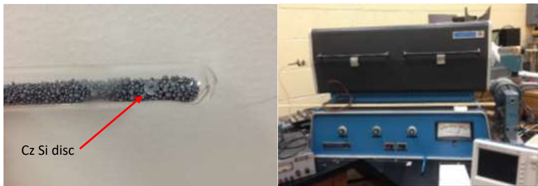
Figure 4.1: Cz Si disc in clean quartz tube surrounded by small Si balls (left). The oven in the Advanced Physics Laboratory used for annealing specimens (right).
