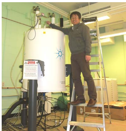
Dr. Rensheng Luo works with the new Agilent DD2 600 MHz NMR spectrometer
