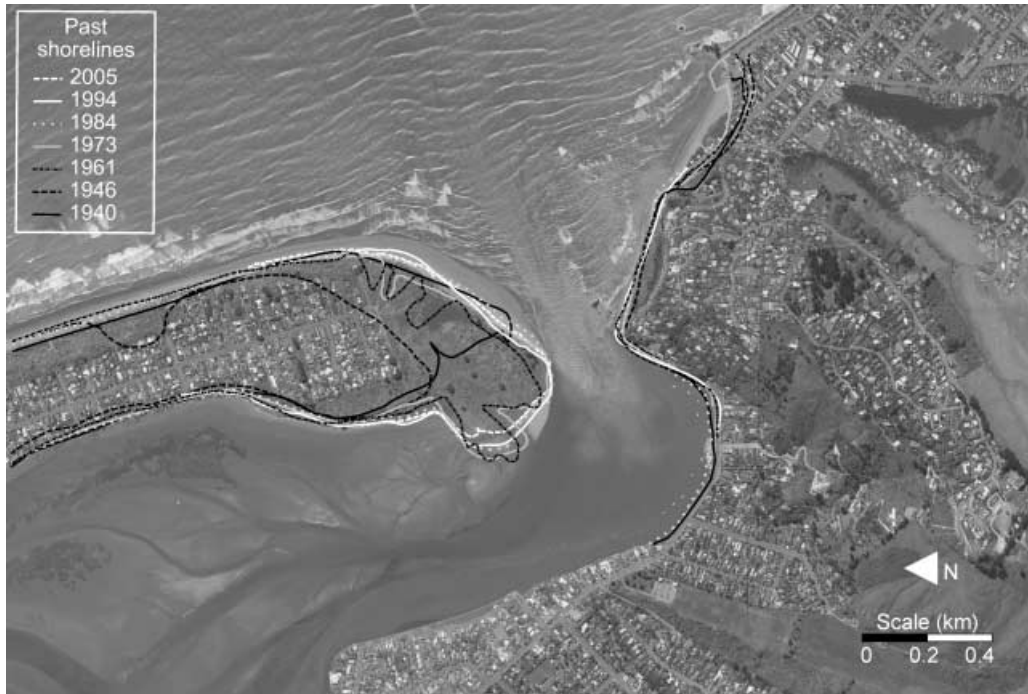
Figure 6 Shoreline changes along the distal end of New Brighton spit 1940–2005 (modified from Hart et al. 2008).
