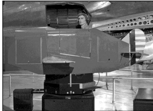
Figure 5 The Link Trainer used for practicing instrument flying. USAF photo in the public domain.
