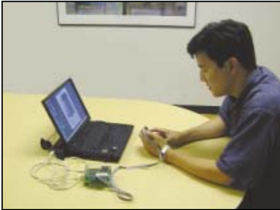
Figure 7. Buck user testing. A participant holds the functional model in his hands to control the animation on screen. The device is tethered to a laptop for usability testing in various locations.
