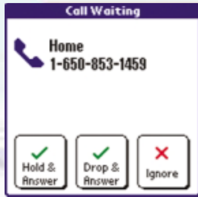
Figure 3. Screen prototyping. Screens are animated in PowerPoint using invisible buttons that allow for simple branching of navigation. The designer can use the buttons to click through different paths, allowing the test driving of specific ideas as well as sharing within the design team.
